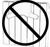
The radiator must be installed to the wall with the provided mounting bracket.
